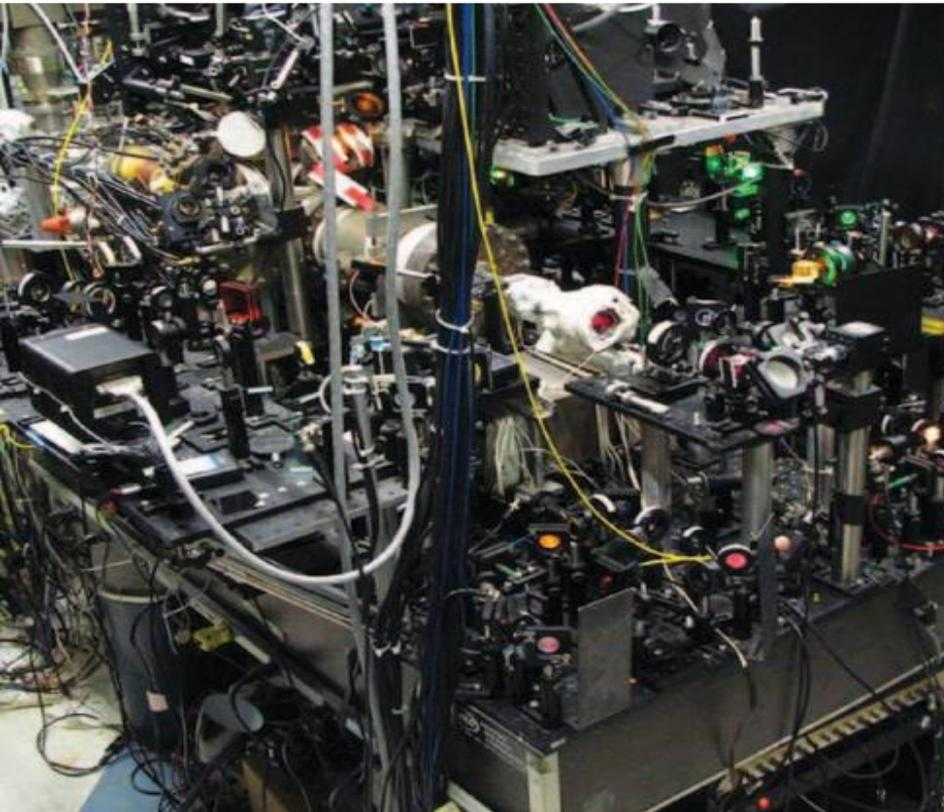
Vacuum chamber, countless mirrors, magnetic coils, water cooling, CCD cameras and lasers for laser cooling of atomic gases (human size)
